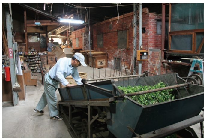
Figure 10 Drying furnace for Matcha tea processing in Uji City (©Kyoto Prefectural Agriculture, Forestry and Fisheries)
