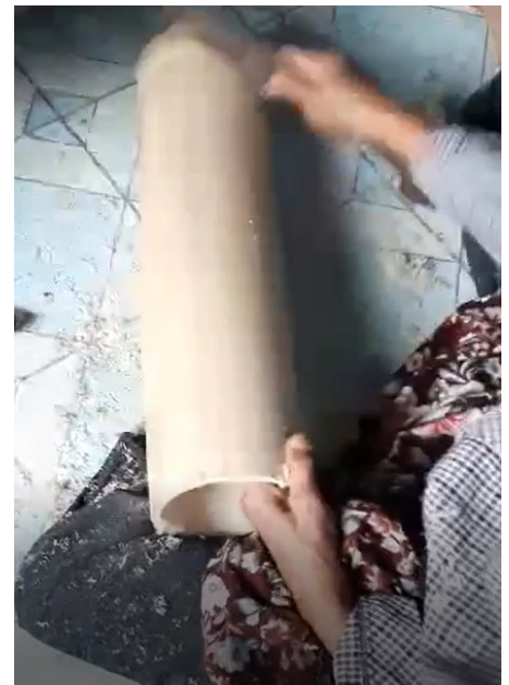
Scraping the bamboo and smoothening it prior to the designing process.
