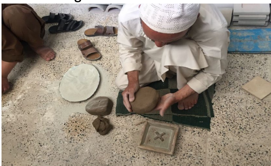
7. Molding the tiles
