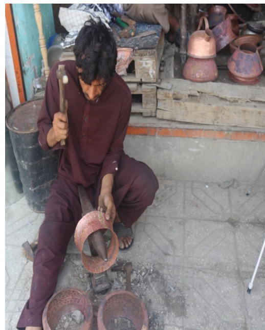
Hammering stage to make copper-made tools
