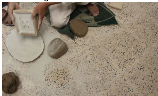
8. Covering the molds with dry dust to prevent tiles from deforming when they are removed from the molds
