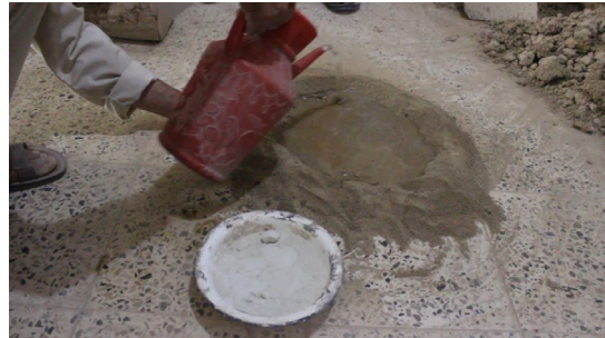
4. Adding water on the soil
