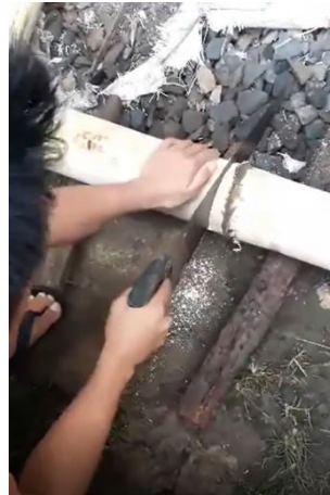
Photos:(Left) Scraping of the outer green layer of Tamlang; (Middle) Drying the bamboos under the sun; (Right) Cutting the bamboo post to desired sizes.
