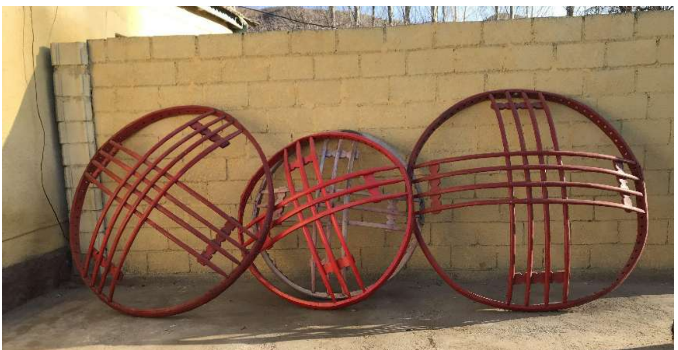
Round frames for the yurts' roof – "tündük" in the workshop of a yurt-maker in Kyzyl-Tuu village
